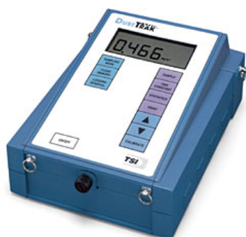
Rys. 12. Fotometr DUST-TRAK Aerosol Monitor, TSI model 8520
